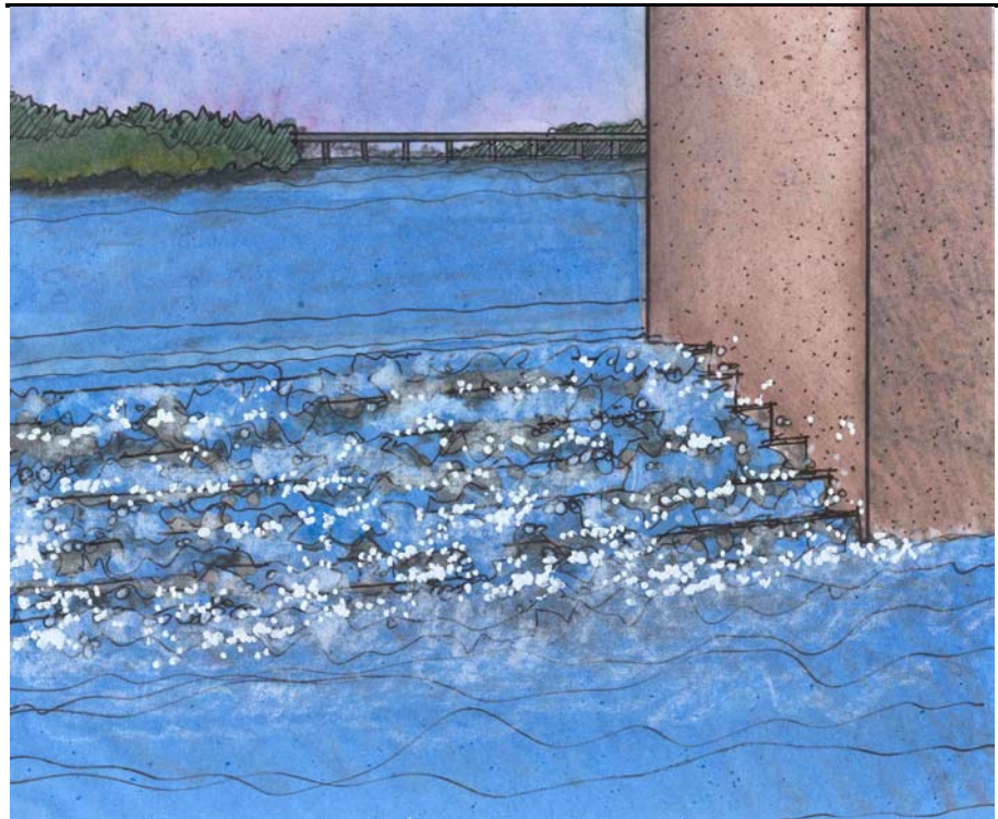
Conceptual sketch of water riffling over a cascade weir section
